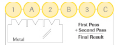
Final result is a combination of using 3 heads T-D-P and 3 heads drive cleat through two passes.
