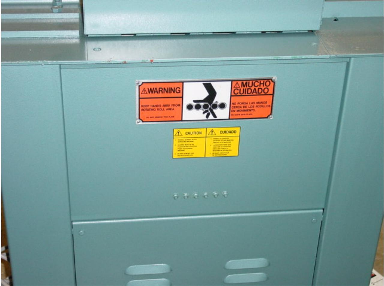
3. Never clean forming rolls while rolls are rotating—turn power off to clean rolls.
