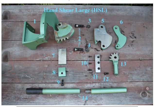
Hand Shear Large (TK No. 2 Hand Shear)
